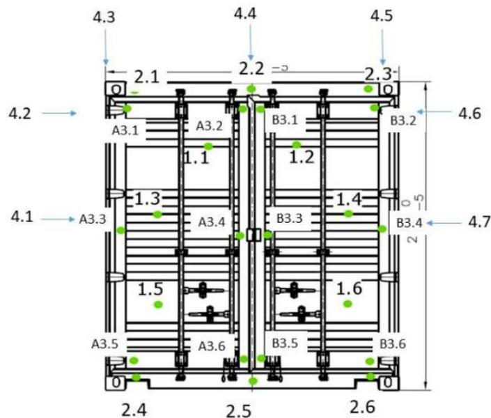
Figure 18 – Thermocouple placement on door
