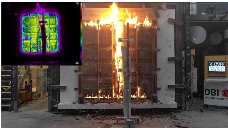
Figure 23 – Ignition of rubbers seal around doors at 17minutes
