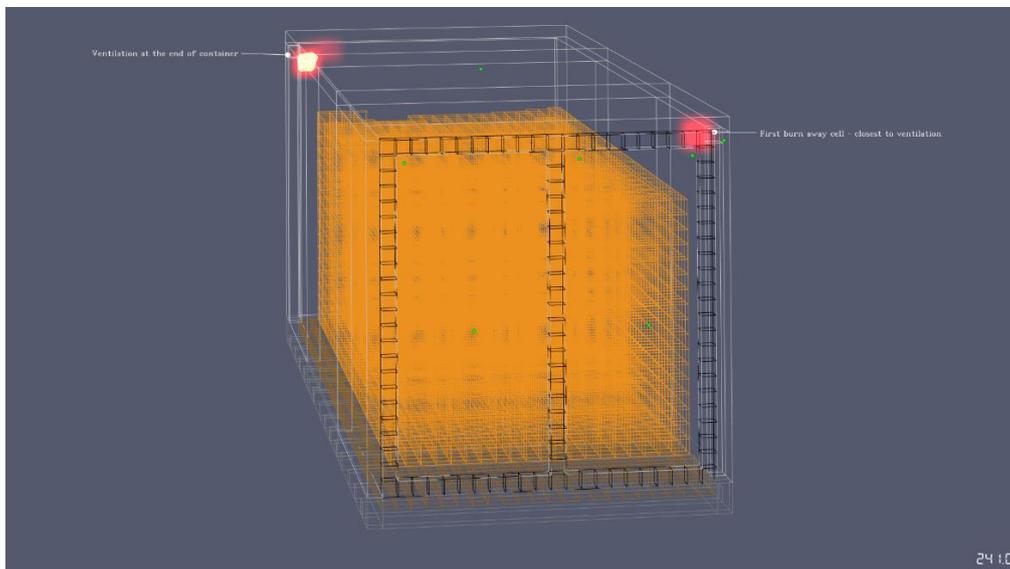
Figure 40: Fire at the ventilation holes
