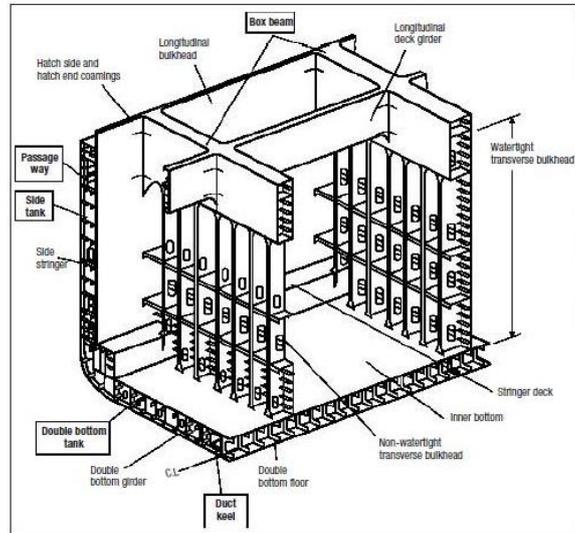
Figure 35 – Usual cargo hold configuration for container ship
