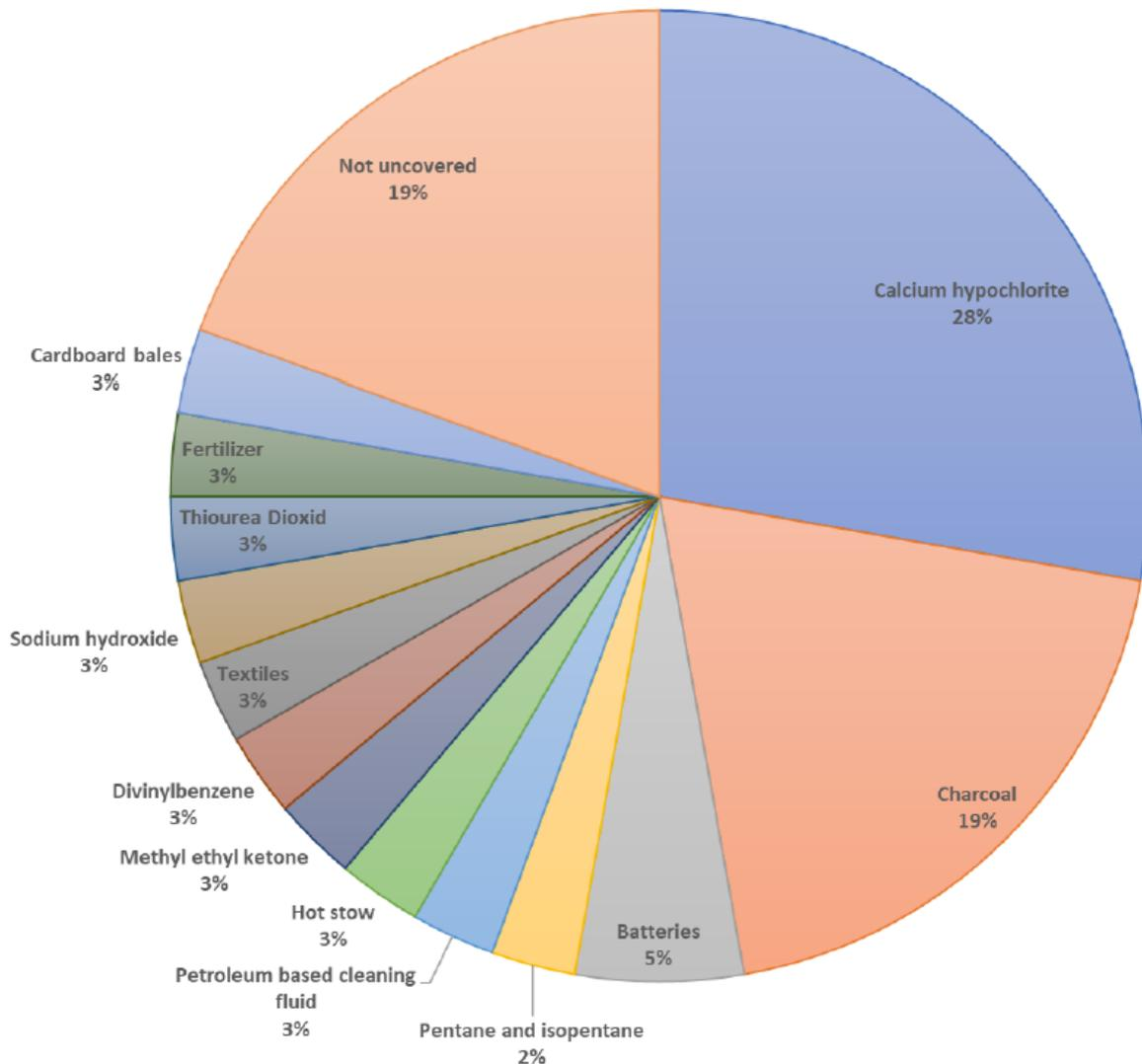
Figure 3 - Causes of fires on board cargo ships in %
