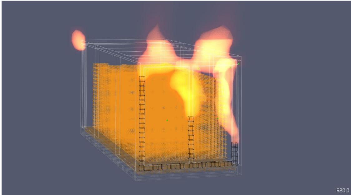
Figure 41: Burn away of the door gasket
