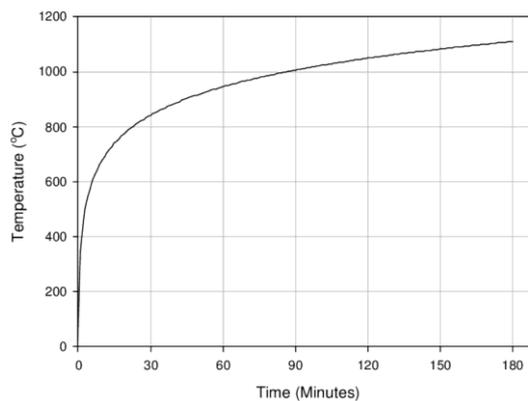
Figure 17 – ISO 834 standard fire curve
