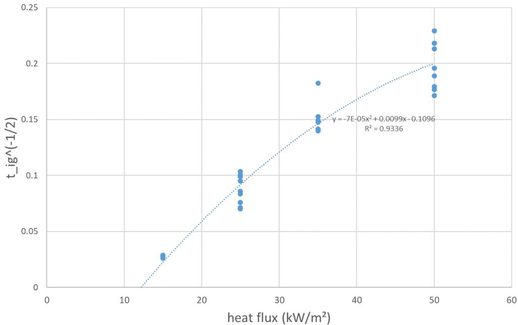
Figure 24 – Determination of Critical Heat Flux
