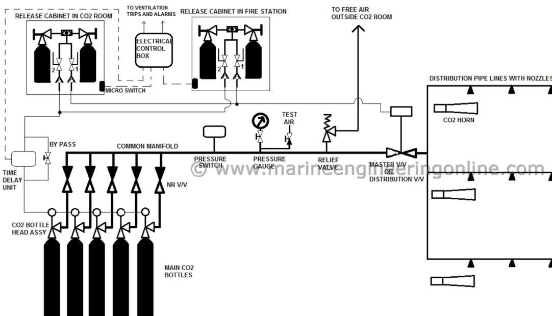
Figure 48: showing diagram of a CO<sub>2</sub> flooding system
