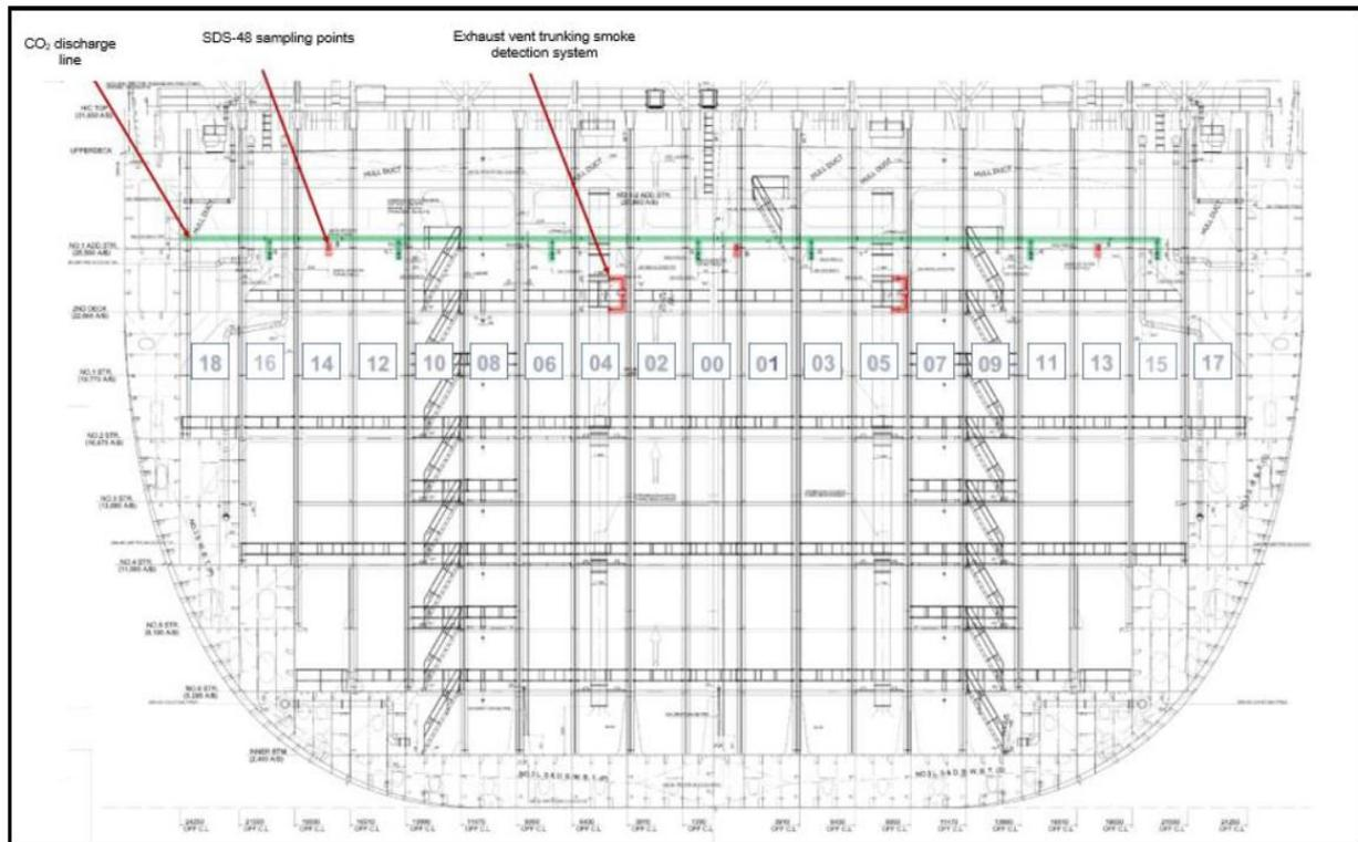
Figure 49: Showing the pillar bulkhead of cargo hold 3 in MAERSK HONAM (picture taken final incident report)
