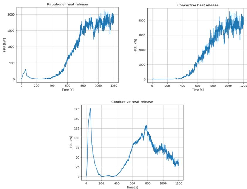
Figure 47: Composition of HRR from the three main elements
