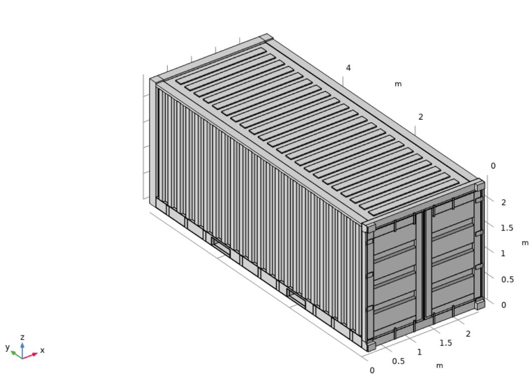
Figure 26 - Geometry of a 20 foot container (snapshot from DBIs model in COMSOL multiphysics)
