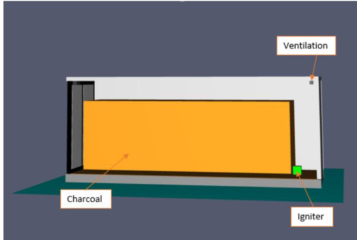
Figure 31: Container content and igniter
