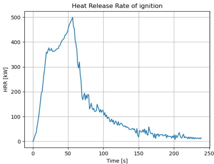
Figure 37: Graph of the HRR during ignition in container
