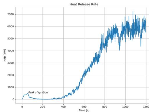
Figure 46: Total HRR during the simulation time
