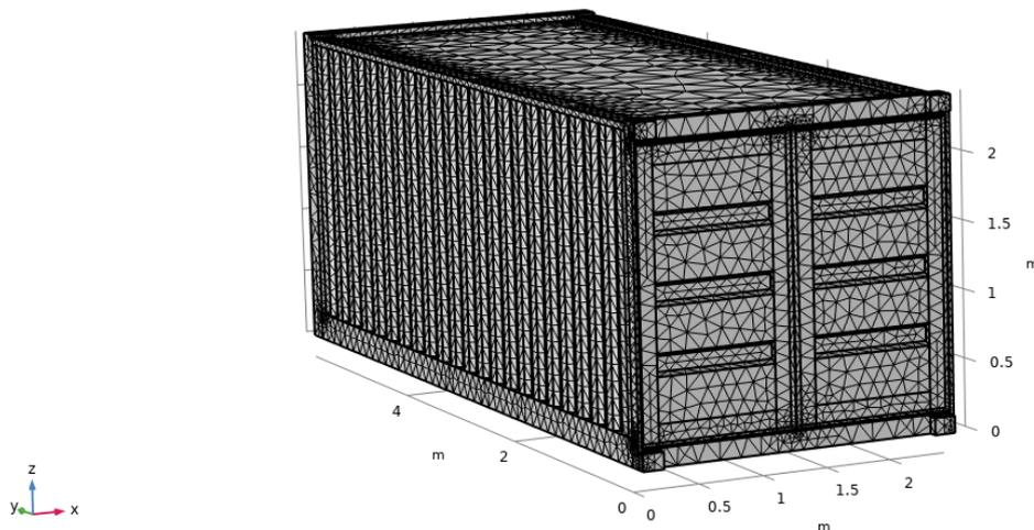
Figure 27 - Meshed container using shell and solid 3D elements
