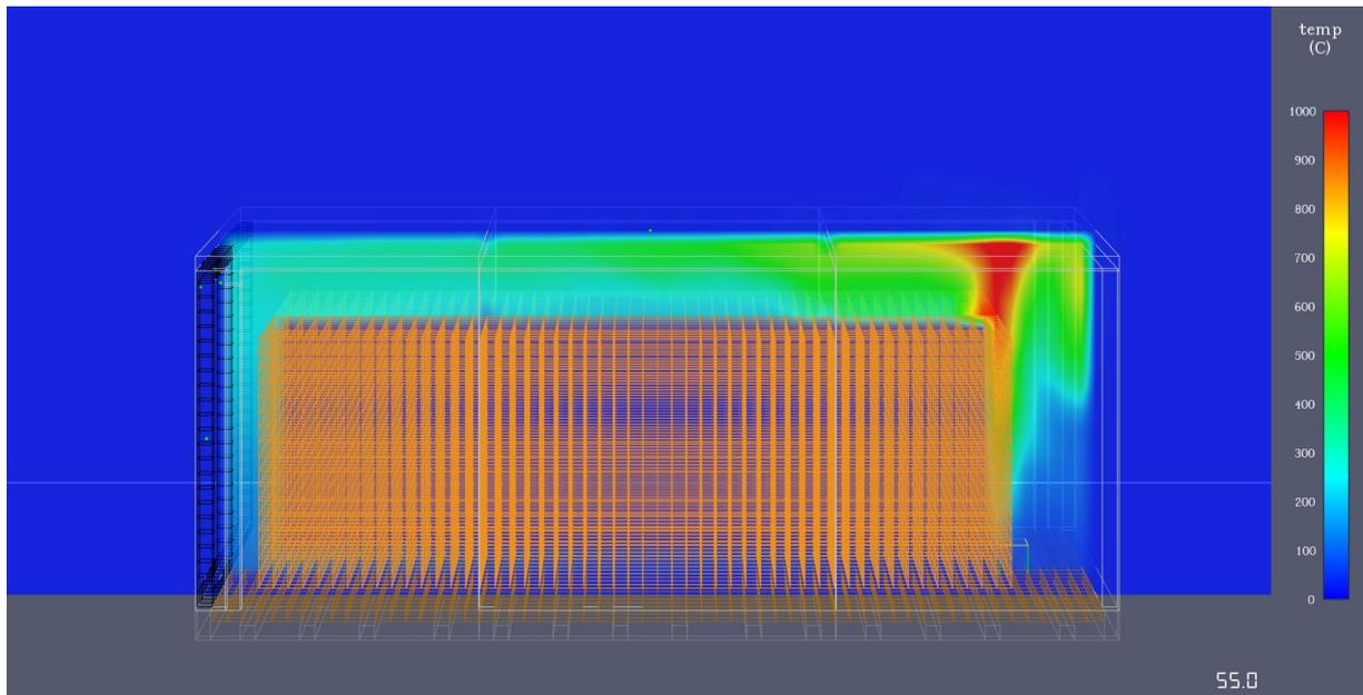
Figure 38: Temperatures along the middle of the container during ignition
