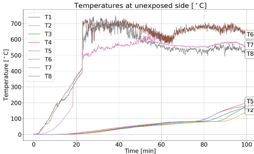
Figure 21 – Temperature reading from the mobile furnace test
