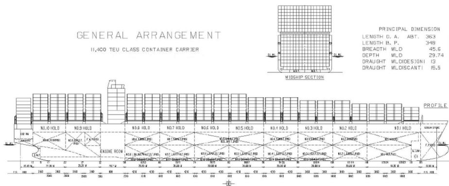
Figure 33 – Mid ship section and characteristics of the container ship used for the modelling work
