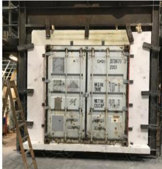
Figure 16 – Door mounted on furnace
