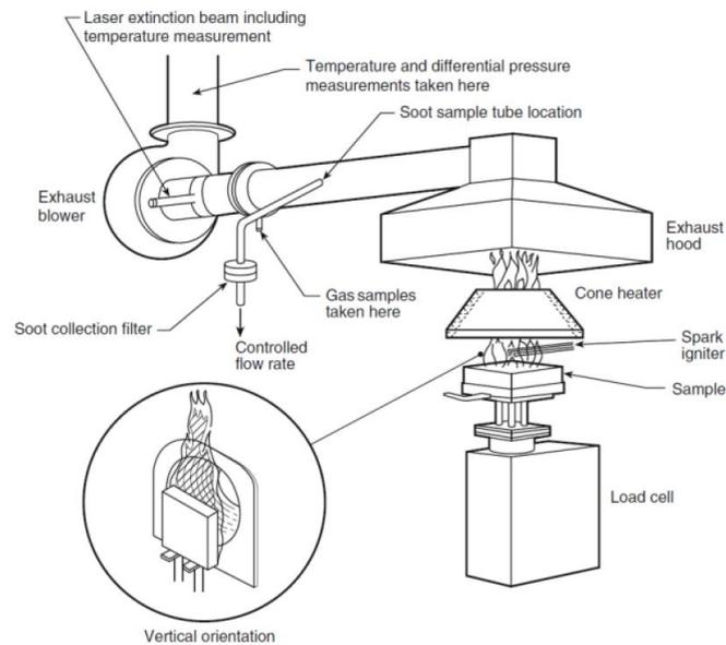
Figure 8 – Schematic of cone calorimeter apparatus
