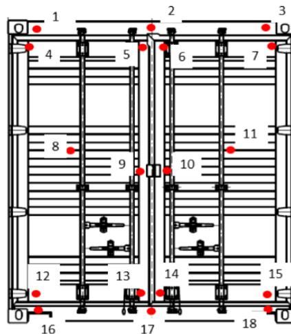
Figure 19 – deflection measurement point placement
