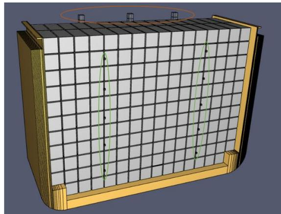
Figure 36 – FDS model of the cargo hold, showing ventilation inlet and outlet
