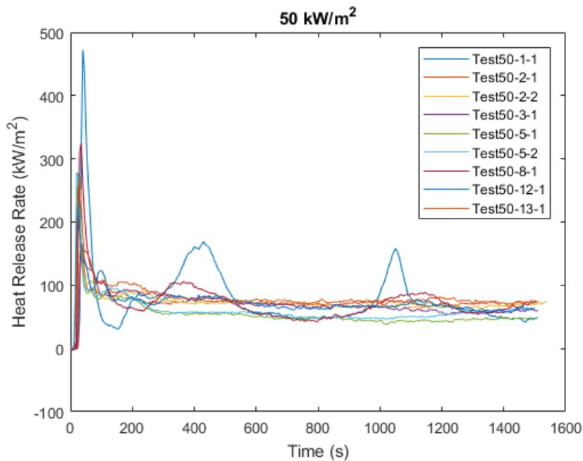
Figure 20 – heat release rates for all samples tested at 50kW/m2 incident heat flux.
