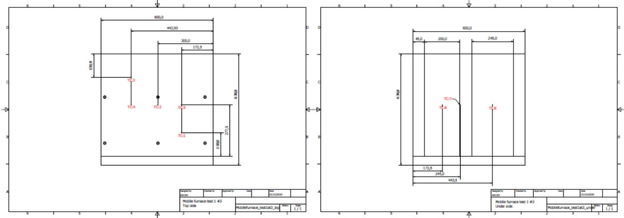
Figure 14 – Thermocouple placement
